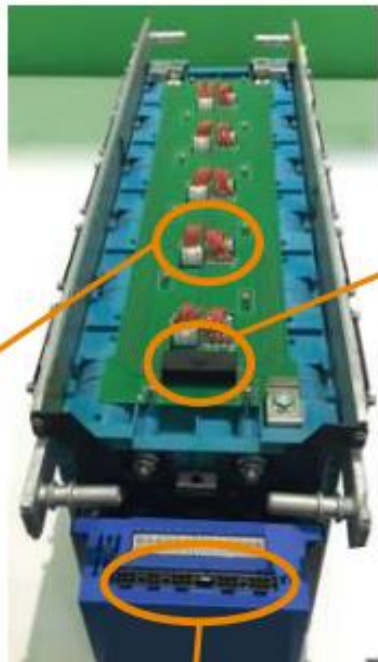
Transfer signal between battery cell and mainboard D1000/D3000
